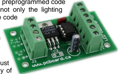
ribbon. The processor is reprogrammable with your own sequences providing you have an inexpensive programmer setup capable of programming the PICAXE 08-M.
