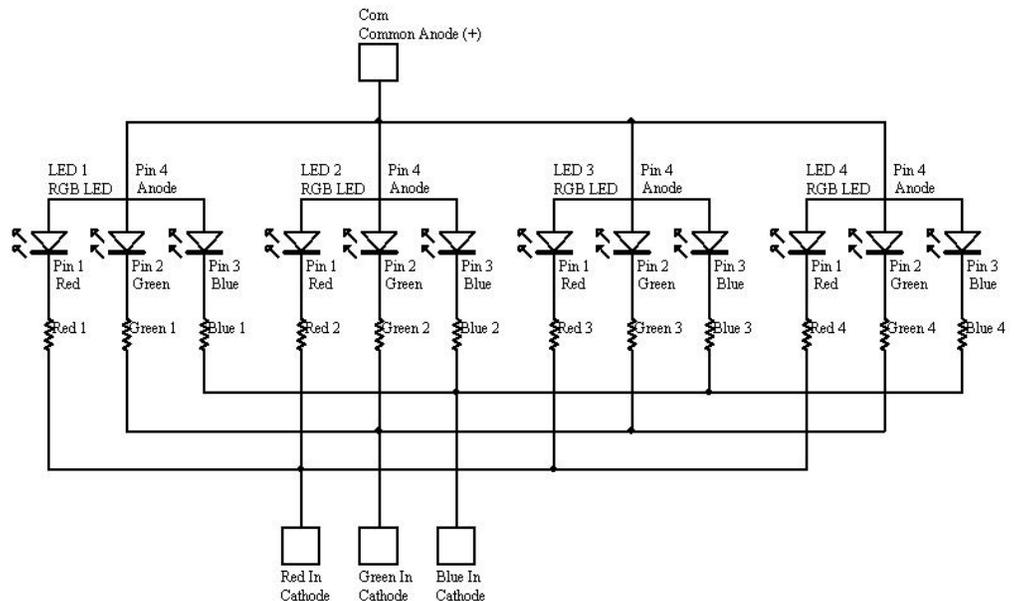
The value of the current limiting resistor is determined by the supply voltage to the circuit, the voltage drop across each LED and the current desired through the circuit. As a rule, keep the current through each leg of the circuit to approximately 20mA to 25mA, which is normally the standard for LEDs. The chart below will assist you in determining the correct dropping resistor needed for your specific application.
