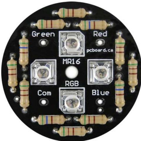
The eight 510-ohm resistors will go be mounted on the board in the “Green” and “Blue” resistor locations, while the four 560-ohm resistors go to the “Red” resistor locations.
