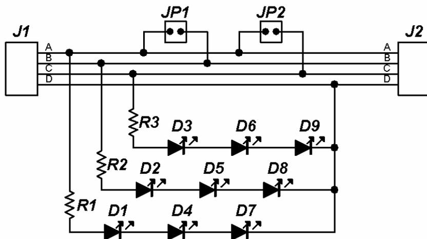
Another exclusive feature of the **LED Lite** board allows you to chain the output of one board to the input of another. Connect the "A", "B", "C" and "D" outputs on one board to the corresponding inputs on the next board. The "A", "B", "C" and "D" connections are connected straight through on the board so either end can be an input or output to connect to the next board. Care should be taken to only connect up to a maximum of four boards in the manner.
